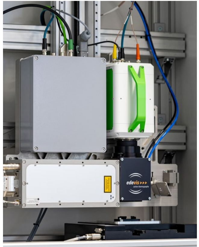
Figure 4: INSIGHT-L inspection head with active pilot laser
