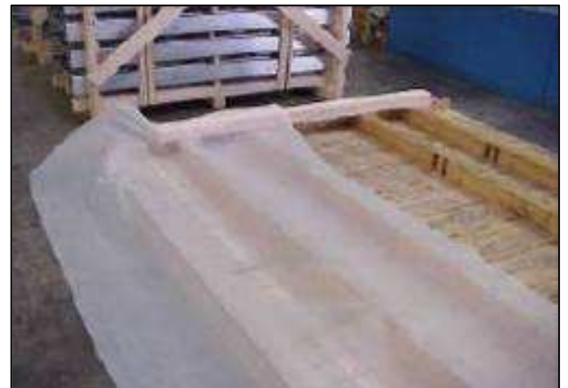
To protect the platform from the VCI film, line it with cushioning film.
