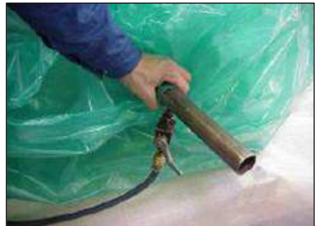
A portion of the air is evacuated to increase the saturated vapor pressure of the VCI gases. The opening is then sealed (welded).
