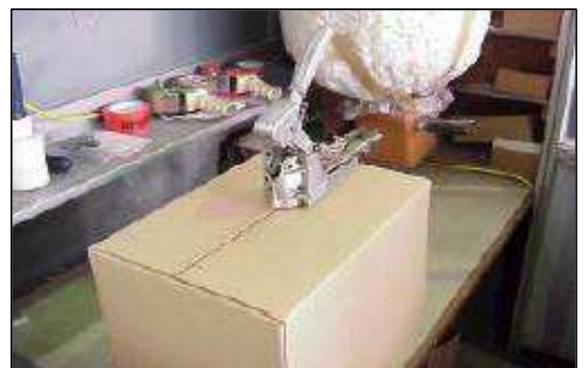
For heavier weight, the top must also be stapled!
