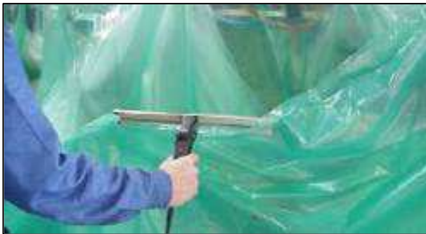
After placement, the film is sealed (welded). (Leave an opening for air evacuation!)
