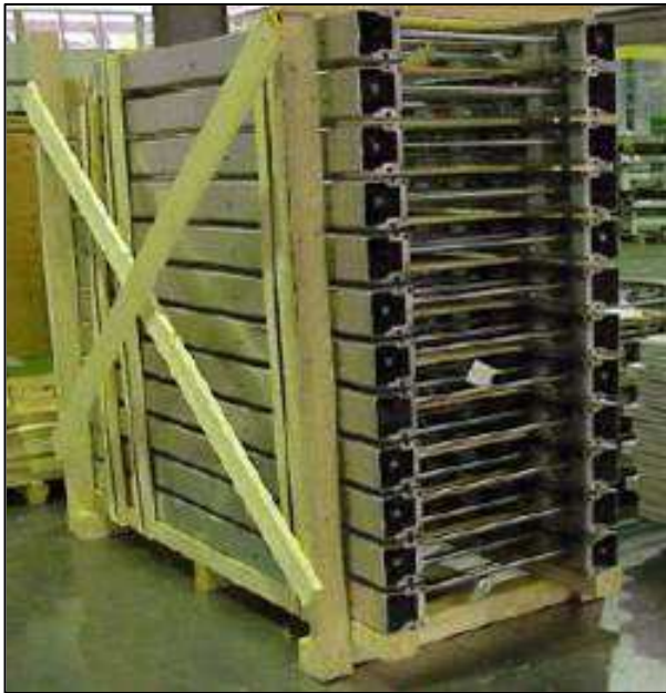
The goods are secured with braces and steel strapping.
