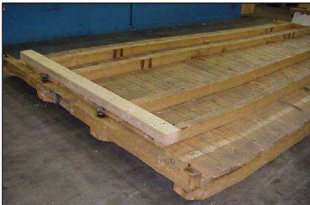
Provision of the platform with support timbers and stop blocks placed on top
