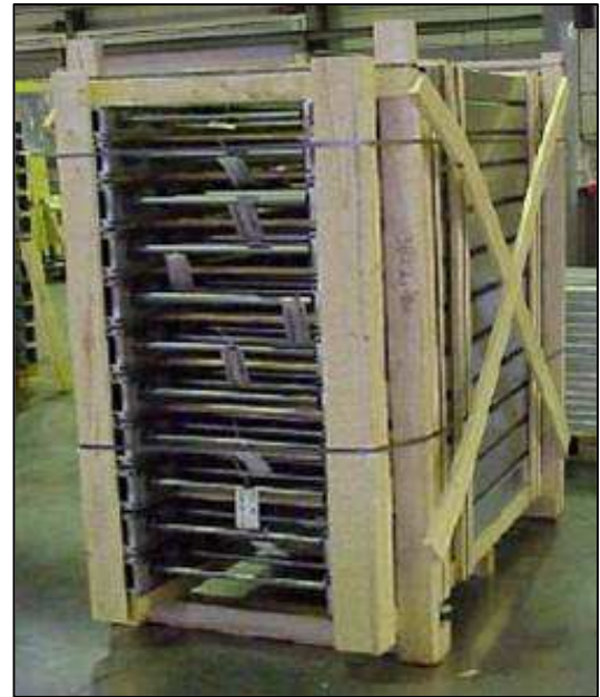
If necessary, the face sides must be protected with boards.
