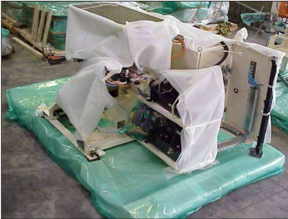
Edges and corners must be covered with protective cushioning film.
