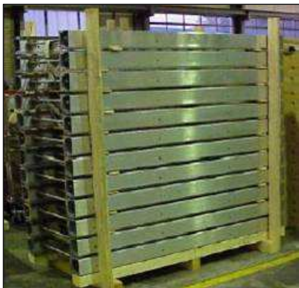
The crates used for packaging FR tracks, transport system stands, safety guards, and other bulky goods are timber frame constructions made of squared lumber.
