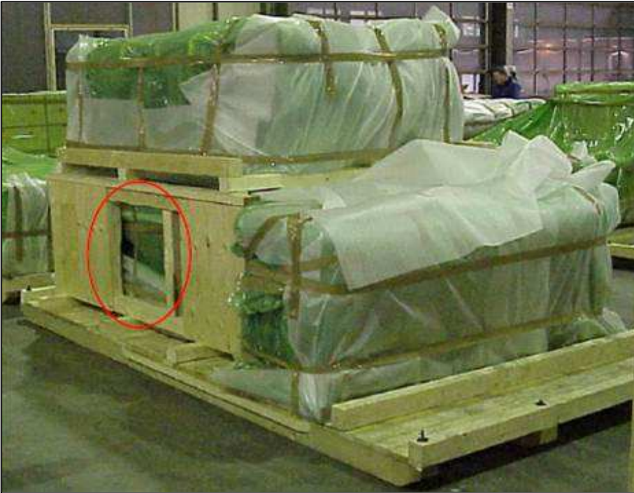
Stable substructure (support frame) made of 10 cm × 10 cm timbers
