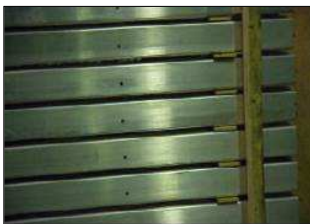
Careful stacking with intermediate timbers
