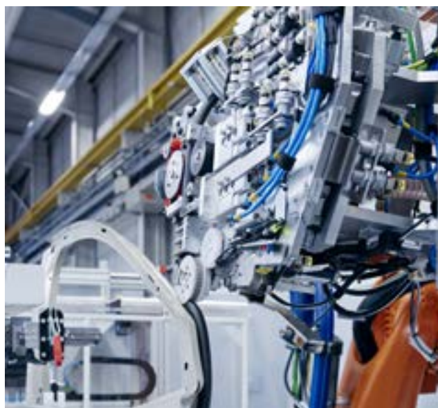
Roll-on unit of the robotic seal application
