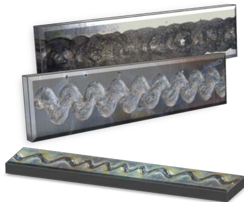
Sinusoidal seam by use of scan unit
