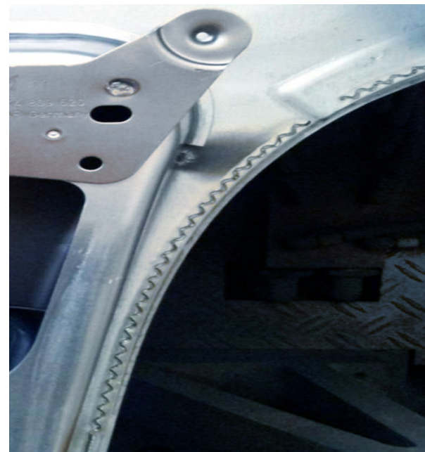
Sinusoidal seam on a part
