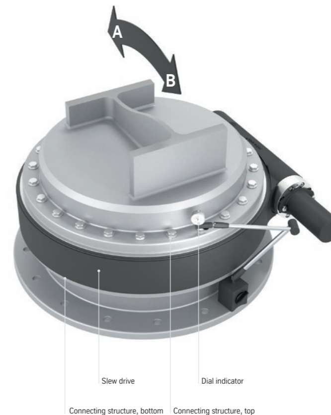
Figure 4: Schematic depiction of tilt clearance measurement
