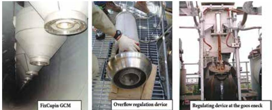
EnviBAT™ Pressure Regulation System- Arrangement Schem at ic and components.
