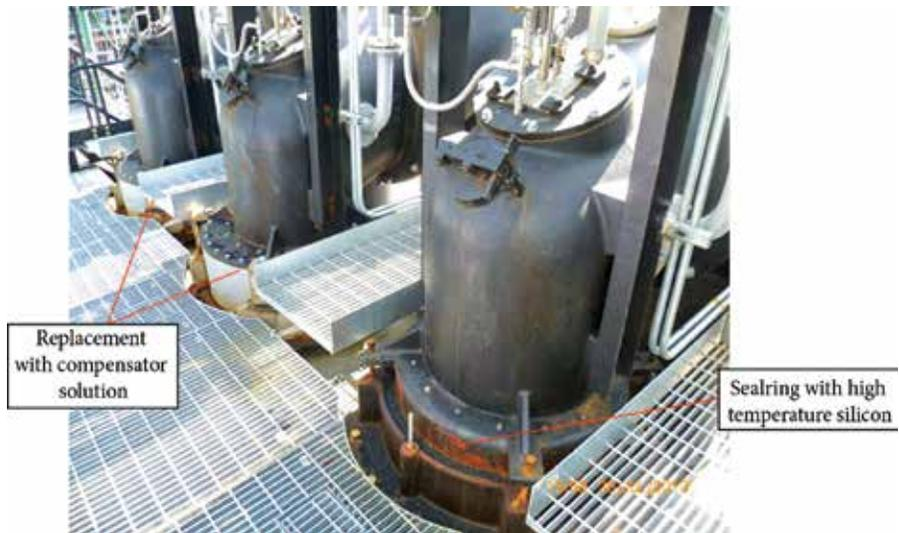
The new compensator solutions. dip pipe sealing in Hyundai Steel Co., Battery 6, South Korea.
