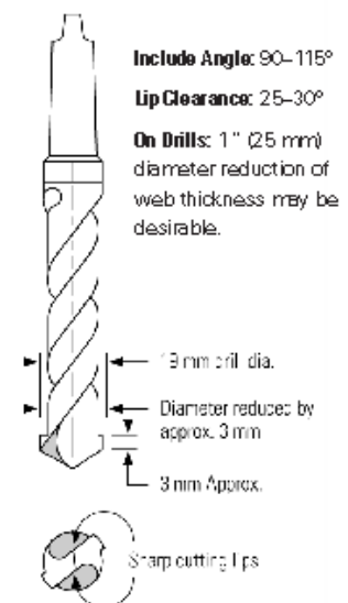
Figure 2: Modified Drill For Vespel® Shapes
