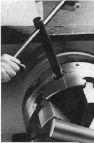
Six-jaw chuck holding cylindrical stock
