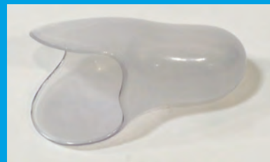
Above: Or-Pro Stiff formed using sprayed water. Below Or-Pro Stiff formed using silicone
