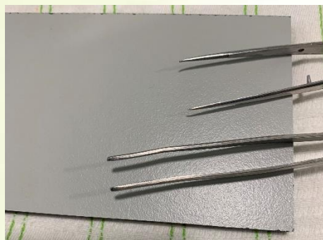
Sharp and blunt tweezers for scratching the surface; scratching only successful with sharp tweezers
