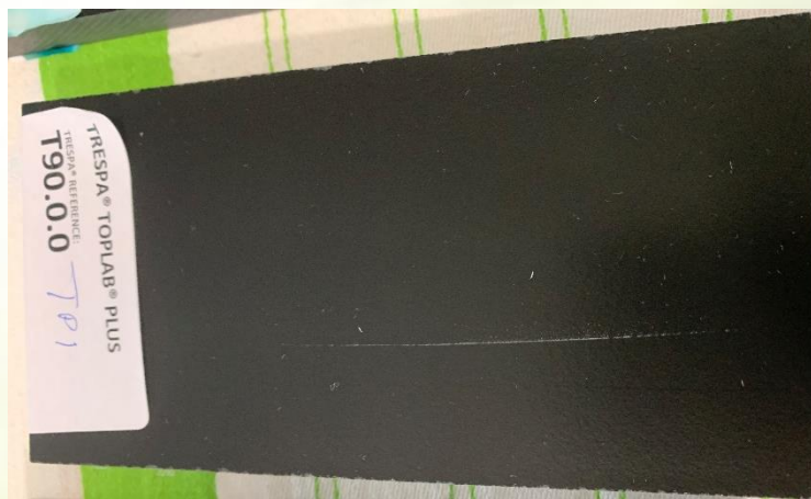
Sharp and blunt tweezers for scratching the surface; scratching only successful with sharp tweezers
