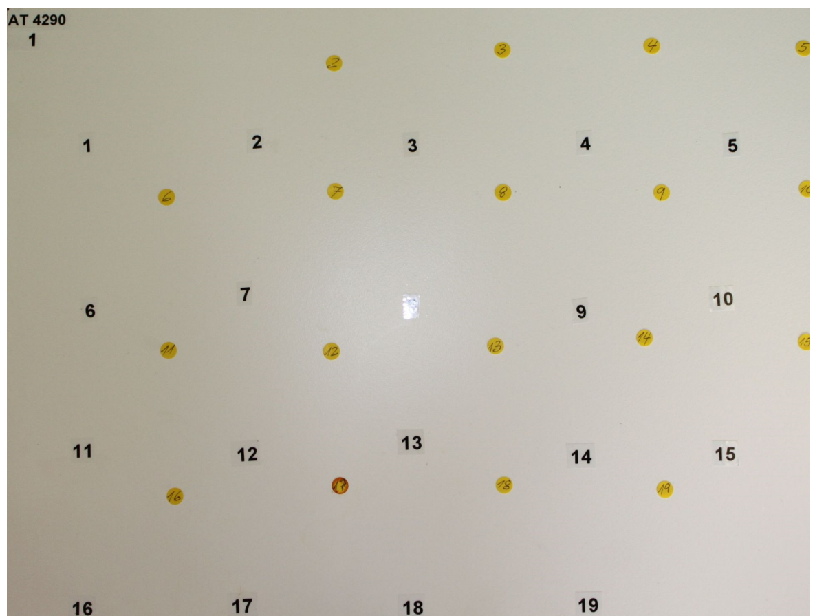
Fig. 1. TopLab ®PLUS T03.0.0 Crystal White after completion of the tests and 48 h drying (wetting test - white markers, drying test - yellow markers)
