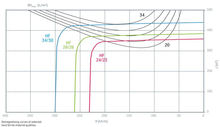
The magnetizing field strength is at least three times the  $H_{cJ}$  value. The relative permeability  $(\mu_p)$  is between 1.05–1.10.
