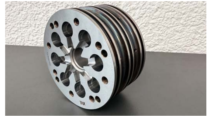
Die holders not installed.
