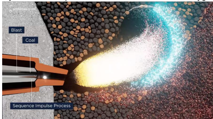
Image 2: Influence of the SIP Raceway effect
