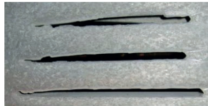
Cast plate after 7,450 operating hours
