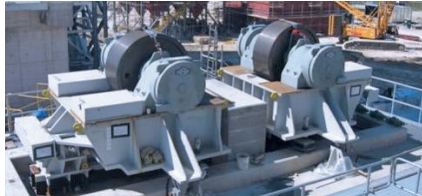
Kiln bearing replacement
