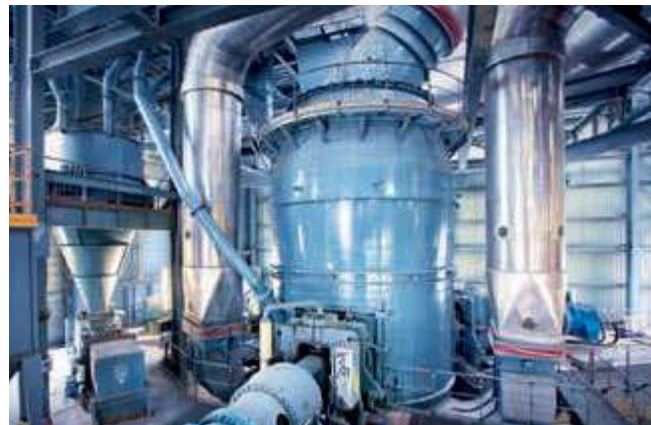
A QMC²-RD mill in France producing OPC finenesses < 10% R 25 µm.
