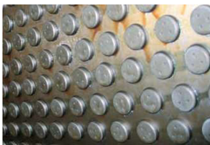
Roll bodies with hard metal studs for low maintenance costs
