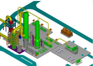
Fig. 3: Envinox® process variant 1: catalytic decomposition of \text{H}_2\text{O} and catalytic \text{NO}_x reduction with ammonia over zeolite catalysts
