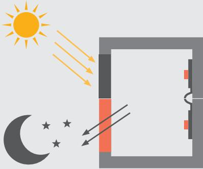
Fig. 1: The principle of the color-change effect
