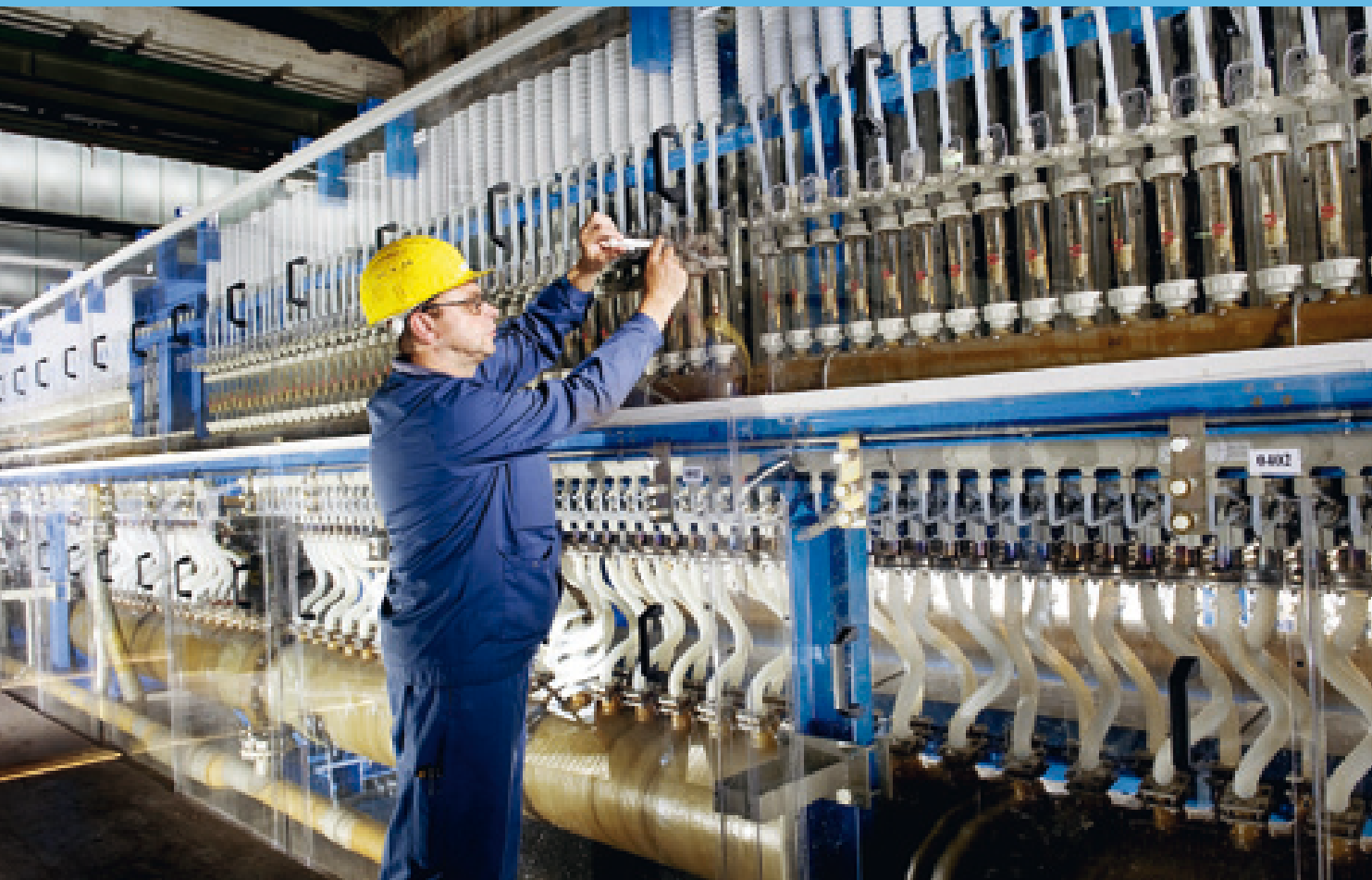
Innovation boosts efficiency: Oxygen depolarized cathodes for the production of chlorine and sodium hydroxide solution.
