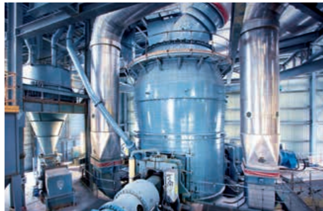
A QMC 2 -RD mill in France producing OPC finenesses < 10% R 25 µm.
