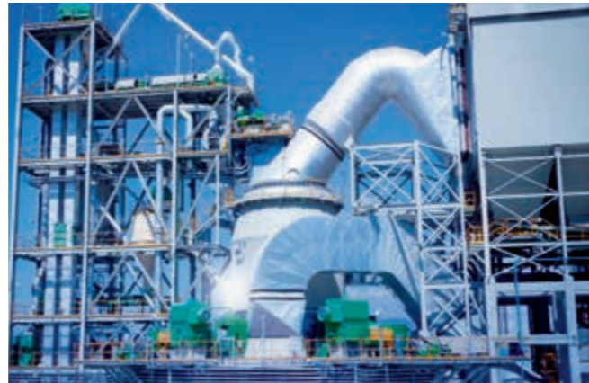
The largest QMC 2 -RD is installed in Mexico. The system has a rating of 4 x 1,800 kilowatt and a capacity of 300 tonnes per hour.
