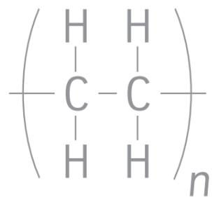
Modern life has become impossible without Low Density Polyethylene (LDPE) and Ethylene Vinyl Acetate (EVA). Photovoltaic cell encapsulation, cardboard packaging coatings, foils, pipes, shoe soles or cable jackets – thanks to its specific physical and chemical properties the thermoplastic material is the basis for products which we meet every day and which are present everywhere.
