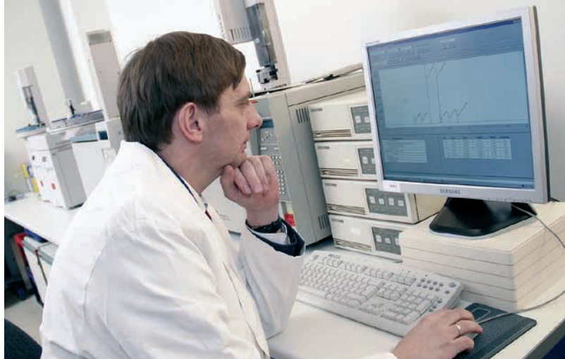
Gas-phase chromatographs used in the separation and quantitative analysis of liquid and gaseous samples
