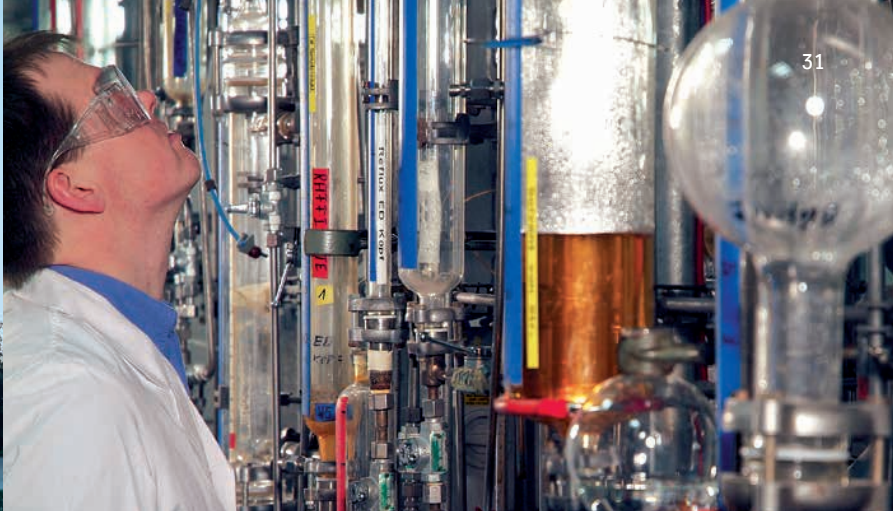
Research facility with PC-based process control system for process development in the fields of distillation, extraction and extractive distillation
