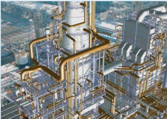
Model of the vacuum distillation unit ( Model der Vakuumdestillation ) Wilhelmshavener Raffineriegesellschaft, Germany
