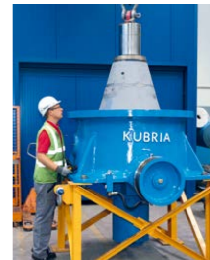
Changing the crushing elements of the Kubria® cone crusher
