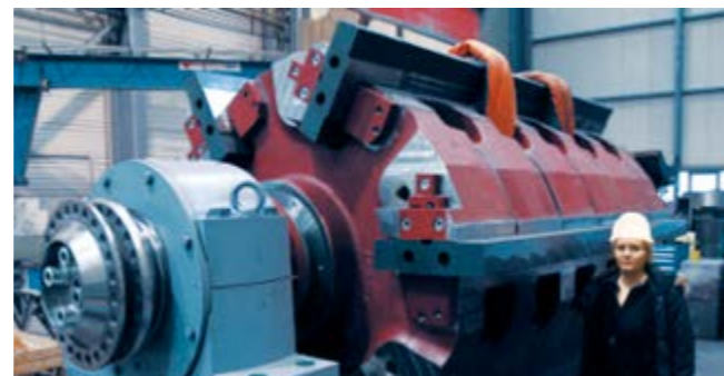
Cast rotor (top) Type PB 200/250 CR Diameter 2,000 mm Width 2,500 mm
