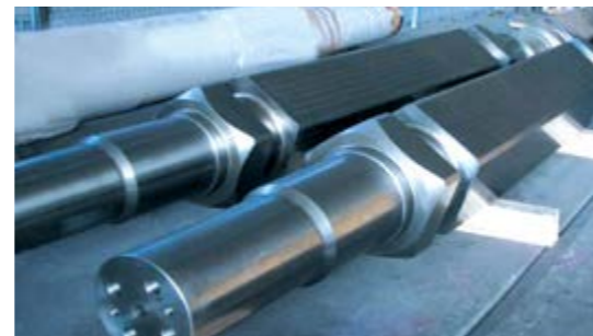
From top: Five-axle rotor for a TITAN® crusher, type 80D160 TITAN® double-shaft hammer crusher with grate basket carrier Pentagonal rotor shaft for a TITAN® crusher, type 60D160
