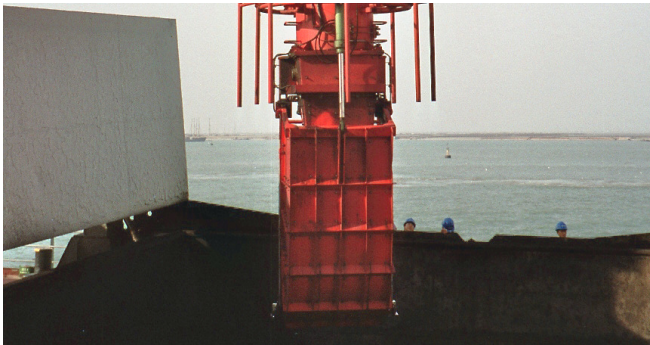
Loading spout with slewable and tiltable trimming spoon
