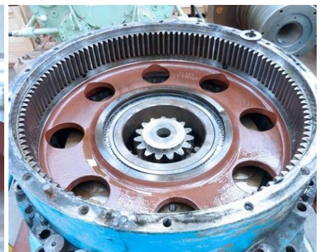
Planetary gearbox refurbishment in the Australia Service Center
