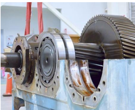
Helical gearbox refurbishment in the Chile Service Center
