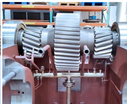
Combiflex gearbox refurbishment in the South Africa Service Center
