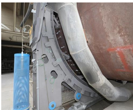
Two separate tensioning ropes for the upper and lower strand ensure easy and uniform pretensioning by steel weights.
