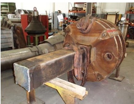
Rotor refurbishment in thyssenkrupp service center Ennigerloh
