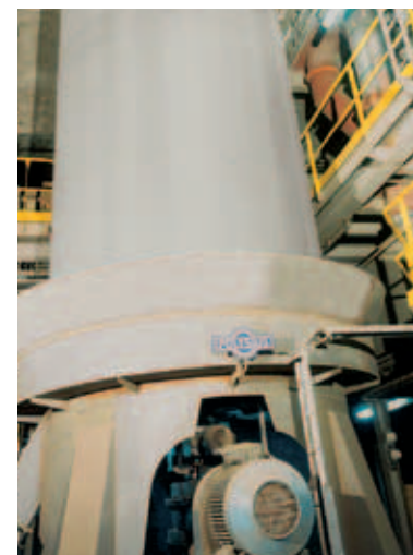
Drive unit of the fines cooler.
