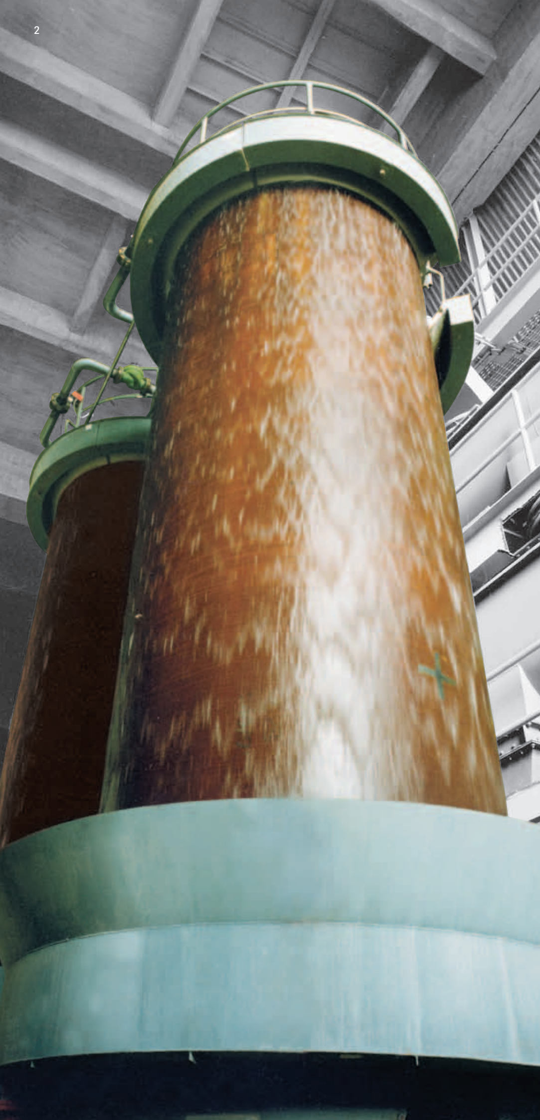
Two fines coolers in a cement grinding plant.
