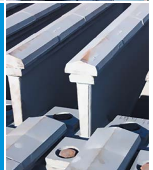
Above: Grizzly screen Type DU-Stk 34 – 3.6 x 4.5 (6.0) ED Screening capacity 7,000 t/h Limestone 0 – 1,500 mm Cut size 140 mm
