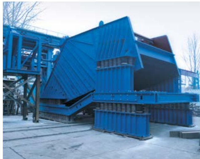
Isolation frame with helical compression springs and rubber buffers
