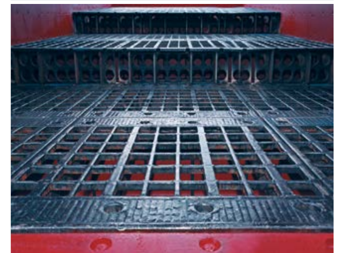
Step-deck linear vibrating screen for oil sand Type DU 64 – 3.6 x 8.0 (8.9) ED
