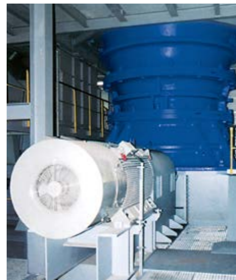
Gyratory crusher with a disc pack coupling, floating shaft and safety coupling
