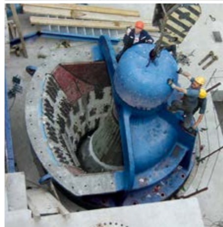
Jaw gyratory crusher for underground iron ore mining and the crushing chamber of a BK 63-75 in a stationary copper ore plant
