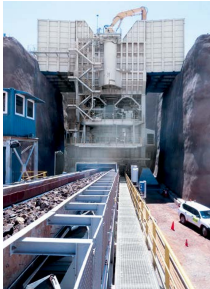
KB 63-89 for iron ore. Capacity: 6,200 t/h
