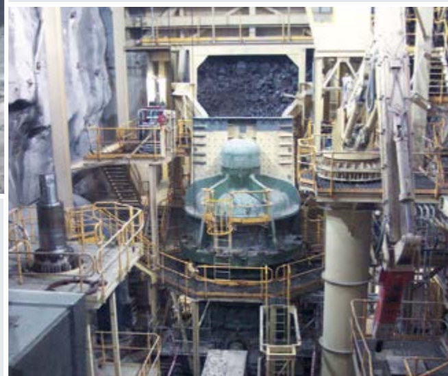
Above: One of two primary crushing plants for iron ore and overburden with KB 63-75 gyratory crusher. The crushers are directly fed from two sides by means of dump trucks.
