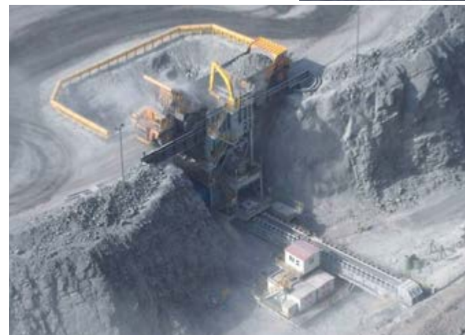
Above: One of two primary crushing plants for iron ore and overburden with KB 63-75 gyratory crusher. The crushers are directly fed from two sides by means of dump trucks.
