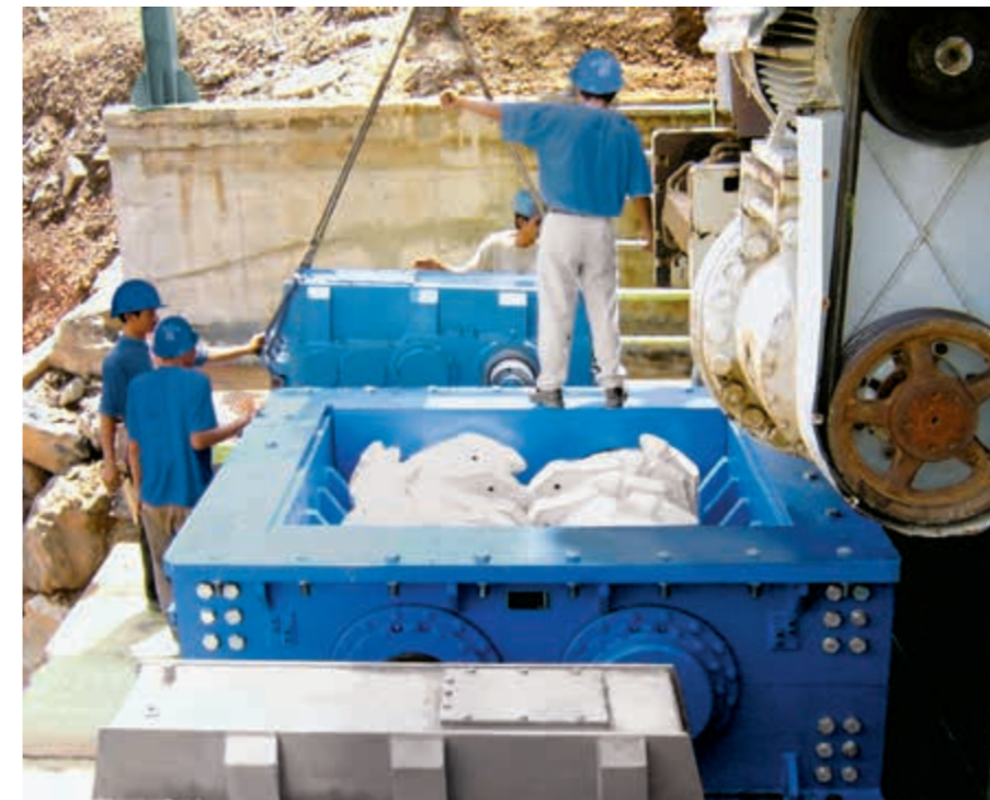
RollSizer, DRS 800 x 1500 CenterSizer, for the primary crushing of silicate rocks. Throughput rate: 700 t/h
