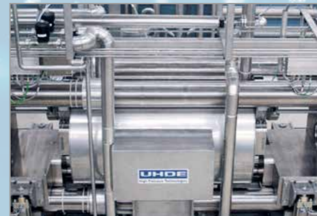
HPP plant / 7,000 bar operating pressure / 121°C operating temperature
