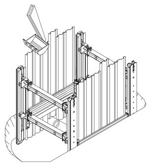
When the sheet piles have been inserted in the two opposite piling frame elements, further soil can be excavated beneath the linear shoring soldiers and sheet piles in accordance with the instructions of project management on site. The sheet piles and linear shoring soldiers are pushed or pressed down in turn. The shoring components must be pressed and on no account struck or hammered.
