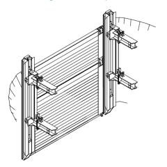
After insertion of the top panels, the shoring unit is lowered with further excavation to the required depth in accordance with the project management's instructions.
