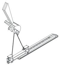
Slide a roller unit into the linear shoring soldier with the aid of lifting gear and a suitable sling (GS-approved). The roller unit's impact plate points towards the top of the soldier.
