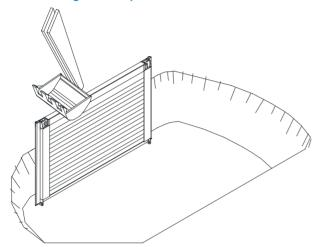
After measurement of the pit, the initial layer of soil is excavated for the shaft to match the panel lengths used. The project management's instructions and the relevant standards must be observed.
