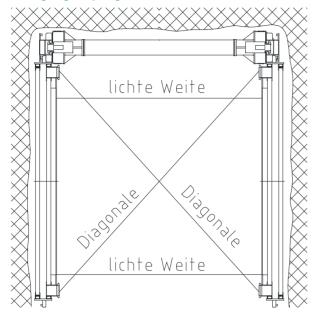
The first shoring unit has to be precisely aligned so that the shoring runs parallel with the trench axis. It is important here that the horizontal clearance between the piling frame element is the same at both ends; and that the two diagonal axes of the shoring unit are the same length.
