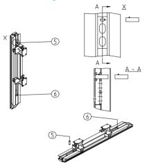
Secure the roller unit in the linear shoring soldier by inserting a pin (5) into the envisaged hole (see detail X) towards the top of the soldier, above the roller unit. After insertion, turn the pin through 180°. At the bottom of the linear shoring soldier there is a fixed stop to limit the roller unit's downward movement (6).
