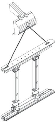
The linear shoring soldier prefitted with the roller units and spacer bars is pivoted over the second soldier so that the roller units and spacer bars can be bolted together.
