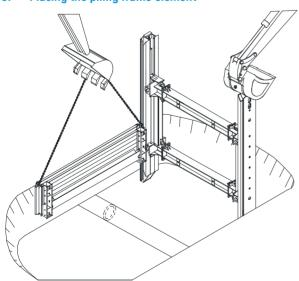
The piling frame element is pivoted from above into the soldier profile (see figure a). Make sure that the rectangular profile (1) on the reverse of the piling frame element catches behind the rectangular profile of the linear shoring soldiers (2).
