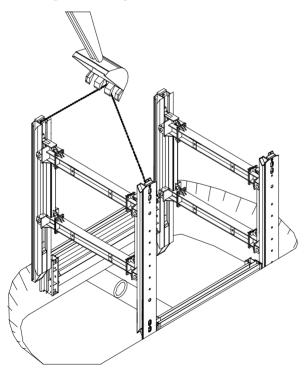
Using lifting gear, the second frame is guided over the exposed guide profiles of the piling frame element and pushed down to the bottom of the trench. On unstable soils in particular, chains must be used to prevent the piling frame elements from sinking.
