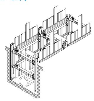
Once the complete desired train of shoring has been fully lowered to the bottom of the trench, pipe laying can start.
