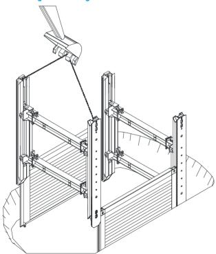
The second frame is guided over the exposed guide profiles of the base panels and pushed down to the bottom of the trench.
