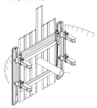
With advance soil excavation in accordance with the instructions of the project management on site, the shoring unit is lowered to its final depth. Chains (GS-approved) are used to lock the waling girders at the horizontal level demanded for reasons of stability. Here, again, the roller unit must be vertically positioned to provide the necessary structural strength (pay attention to length of cantilever).
