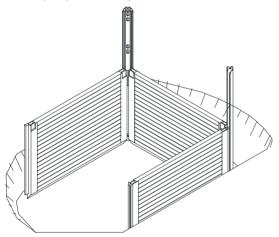
So that the last wall of shoring can also be installed without difficulty, the shoring has to be properly aligned. To this end, it is important here that the horizontal clearance between the shoring panels is the same at both panel ends; and that the two diagonal axes of the shoring unit are the same length.
