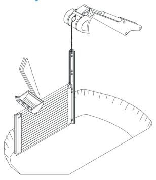
By using a second set of lifting gear, the corner rail can now be slotted in from above. Make sure that the rectangular profile (1) on the reverse of the corner rail catches behind the rectangular profile (2) of the shoring panel.
