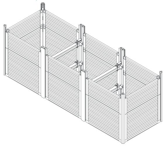
There is no problem combining single-rail linear shoring with corner shoring. This way it is possible to continuously shore pits and trenches.
