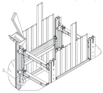
When the pair of linear shoring soldiers has been lowered, both ends of the waling girders rest in the guides of the linear shoring soldiers. The sheet piles are now pressed down. Make sure that the waling girders and sheet piles are pressed tightly together. If the waling girders have to be lowered, they must be prevented from accidentally sliding out of the slide-rail soldiers, e.g. with a chain.
