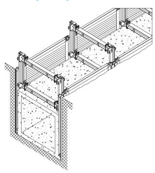
When the concrete walls have set, the shoring is removed in the way described in step 1 in these instructions. If the remaining cavity between the cast-in-place concrete and the soil has to be backfilled, it is essential to use shoring panels and soldiers with integrated injection holes through which a sand-water-cement mix can be injected into the cavities.
