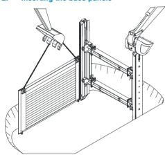
The base panels are inserted from above with lifting gear into the soldier profile (see figure a). Make sure that the rectangular profile (1) on the reverse of the shoring panels catches behind the rectangular profile of the linear shoring soldiers (2). After insertion, the shoring panels are lowered to the bottom of the trench.
