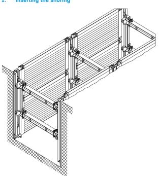
When laying pipes of large diameter or building cast-in-place concrete drains/sewers, additional support for the guide frames at the base of the soldiers is often needed for reasons of stability.
