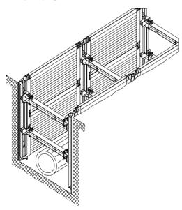
Once the complete desired train of shoring has been fully lowered to the bottom of the trench, pipe laying can start.
