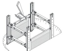
Before the lowering process proper, the soil beneath the shoring panels is excavated in accordance with the project management's instructions. The soldiers, shoring panels and roller units are pressed down in turn, with special use being made of pressure beams for the shoring panels and pressure plates for the soldiers. The shoring components must be pressed and on no account struck or hammered.
