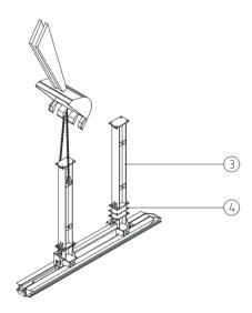
The preassembled combinations of spacer bars (3) required for the desired trench width are aligned with the bolting plates of the roller units and bolted with the required number of bolts as per piece list. To facilitate alignment of the spacer bars during the next assembly step, the bolts are only loosely fastened.
