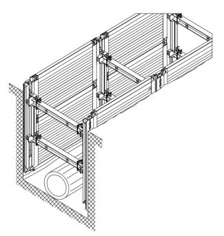
At the end of pipe-laying work, the shoring is removed with layer-by-layer backfilling and compacting. To this end, the shoring is extracted step-by-step in accordance with the instructions of the project manager on site and with the expert's specifications and the backfilling material returned to the trench is compacted against the existing soil.
