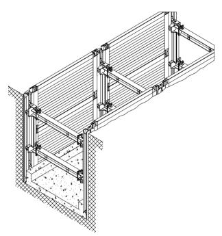
When support for the base of the soldier has been provided, the roller unit can be raised to the maximum permitted vertical pipe clearance for completion of the cast-in-place concrete structure. In this position, the roller unit must be secured with chains or pins.
