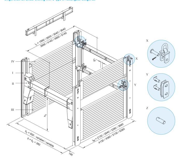
(All dimensions in mm. The details of length of pipe opening  $I_{\rm C}$  refer to the rectangular boogie car.)
