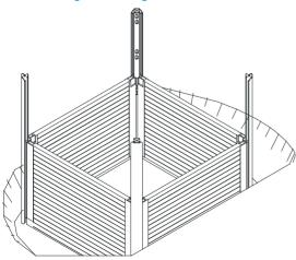
When the fourth base panel has been installed, the rectangularity of the shoring must again be checked. Then the cavity between the soil and shoring panel must be backfilled and compacted.
