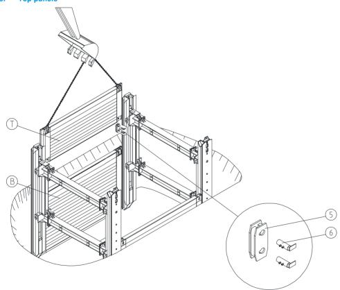
Depending on the required trench depth, the top panels (T) are inserted in the soldier guides when the base panels (B) have been fully lowered.
