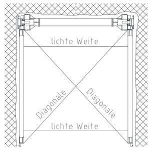
The first shoring unit has to be precisely aligned so that the shoring runs parallel with the trench axis. It is important here that the horizontal clearance between the shoring panels is the same at both panel ends; and that the two diagonal axes of the shoring unit are the same length.
