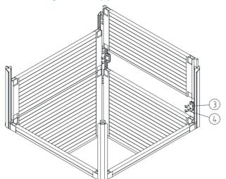
Depending on the required trench depth, the inner top panels are inserted in the soldier guides when the inner base panels (B) have been lowered to the provisional trench bottom.
