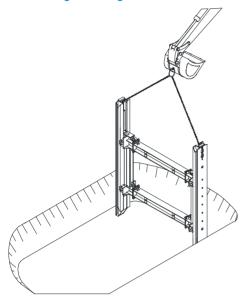
After measurement of the trench line, the initial layer of soil is excavated for the first shoring unit in accordance with the project management's instructions.
