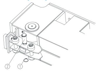
To adapt the U-type roller unit for use in single-rail linear shoring, it is necessary to dismantle the tension anchor. To this end, remove the locking ring (1) with a suitable tool (pliers or chisel). Then pull out the pin (2).
