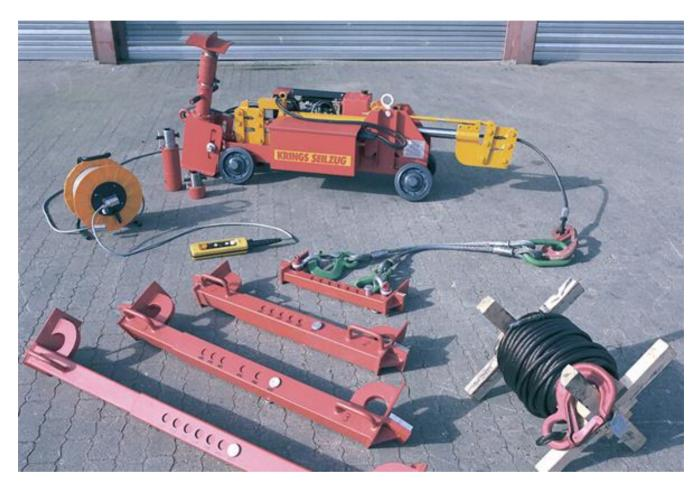
Using the SZ 10 Pipe Puller means that pipe socket seals can be pulled together without damage. Damage to the bed or pipe ends caused by the excavator bucket is also effectively prevented.
