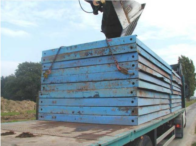
The roadway panels can be delivered to the site location in „packages“ or „one after the other“. For package unloading and for easier handling, E+S generally supplies four S-hooks without charge. With this approved hooks the maximum of six panels may be lifted at one time.
